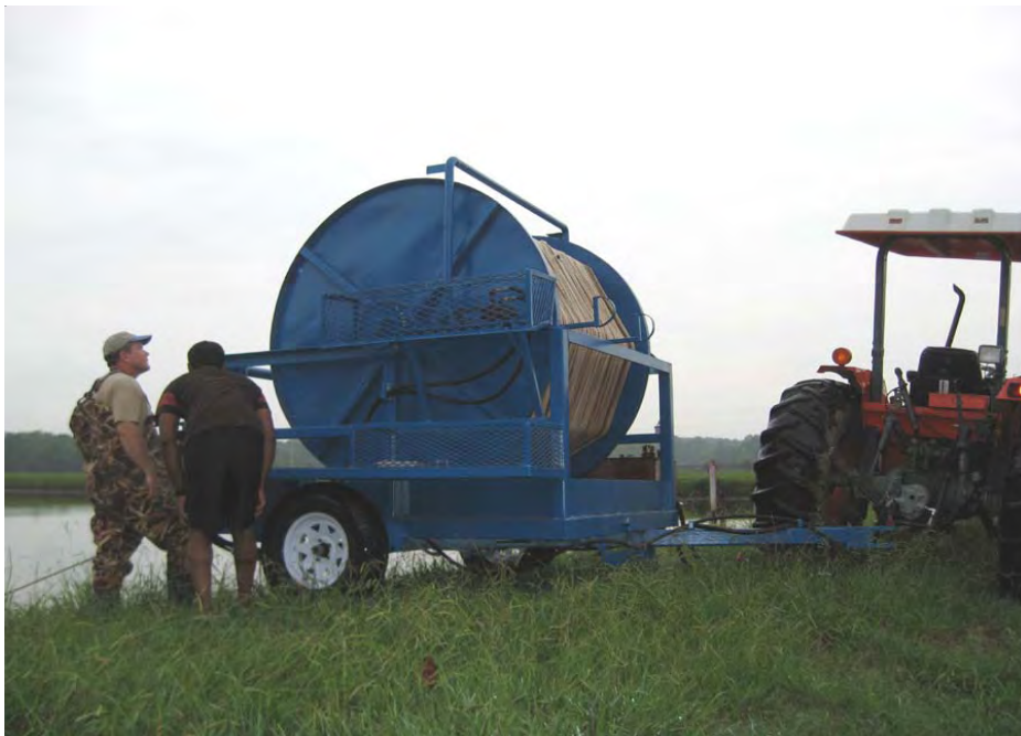
Figure 17. Tractor (43hp) used to pull the trawl using a power take-off driven hydraulic pump.
