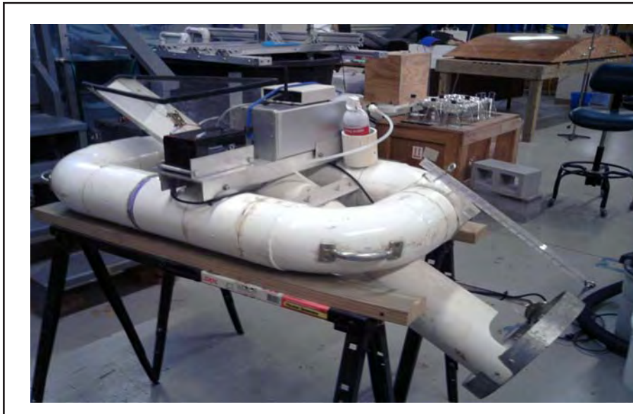
Figure 10. The catfish sizing system with electronics and battery mounted on board and bubbler system in place to provide calibrated signal in data.
