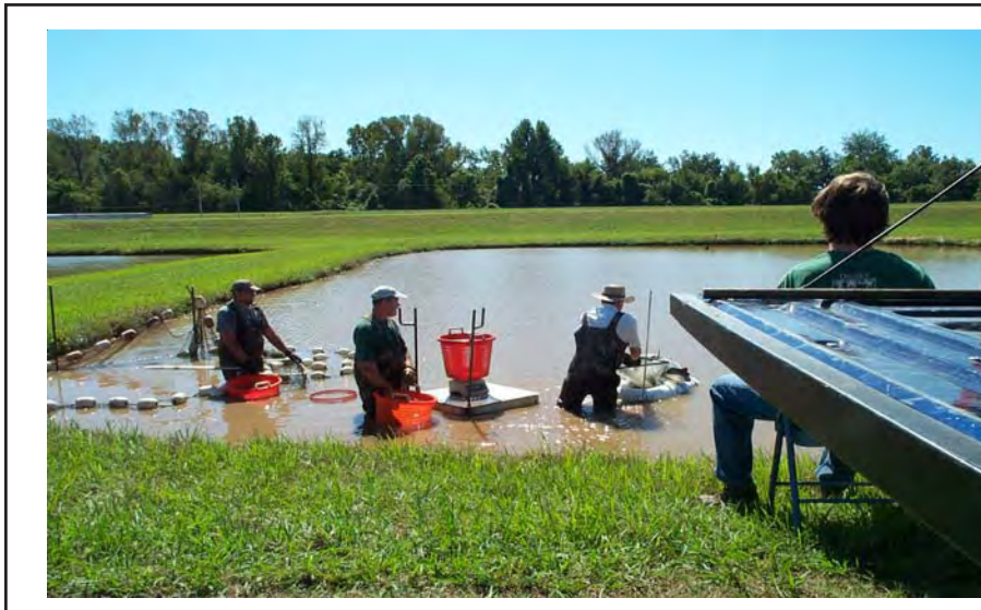
Figure 11. Modified Aquascanner Catfish SONAR system being used to measure individual fish.
